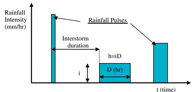
Figure 2. Rainfall scheme of random pulses with random durations and depths mutually independent.
